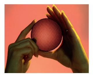
Figure 14: Detail of a catalyst monolith for automotive exhaust gas purification. (© Pixabay / NASA-Imagery)
